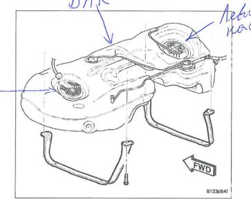
32. Remove bolt for fuel tank strap.
