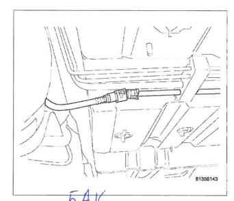
30. Support fuel tank with transmission jack.
